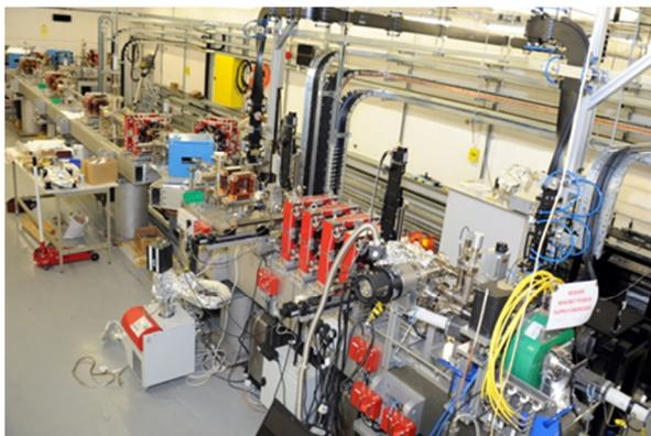
Figure 2: VELA photo-injector module installation.
