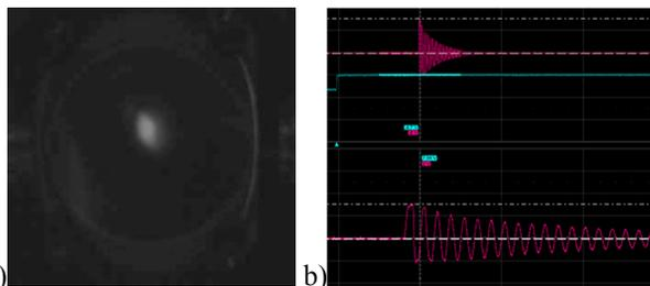
Figure 5: a) First YAG screen beam image and b) signal measured on the Faraday Cup.
