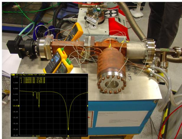
Figure 3: Strathclyde RF Gun, (inset) measured response.
