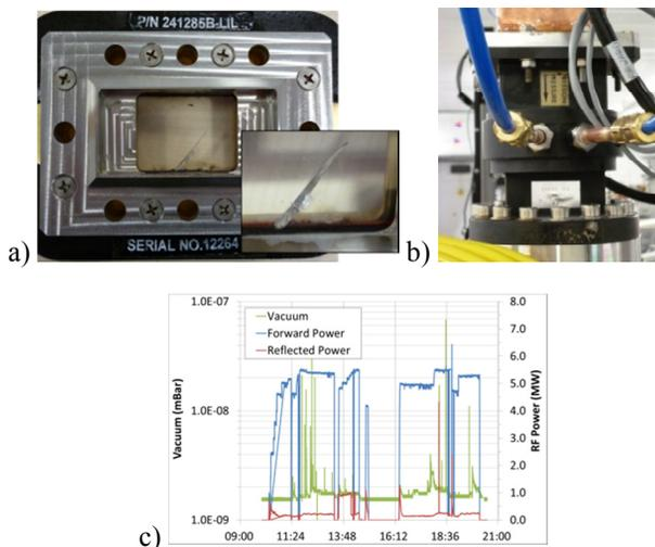
Figure 4: a) Failed quartz window, (inset) window fracture, b) replacement ceramic window and c) RF conditioning results.
