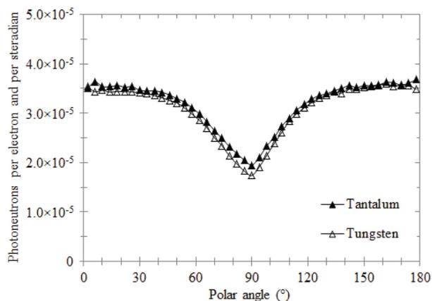
Figure 1: Angular distribution of the photoneutron flux emitted by a tungsten or tantalum target irradiated by 15 MeV electrons.
