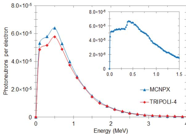
Figure 3: Energy spectrum of the photoneutron flux emitted by a tantalum target irradiated by 15 MeV electrons.
