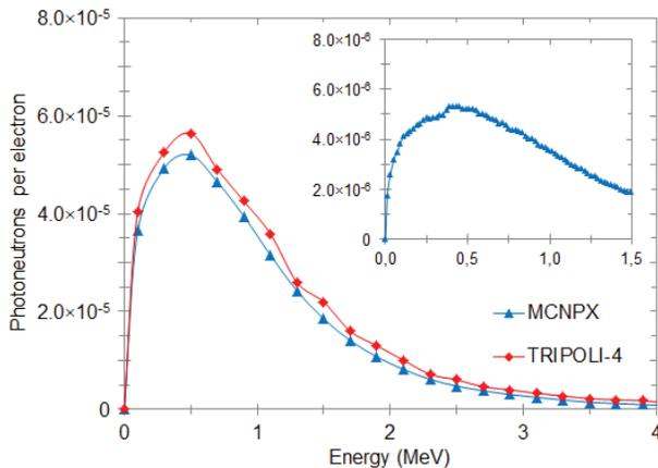
Figure 2: Energy spectrum of the photoneutron flux emitted by a tungsten target irradiated by 15 MeV electrons.
