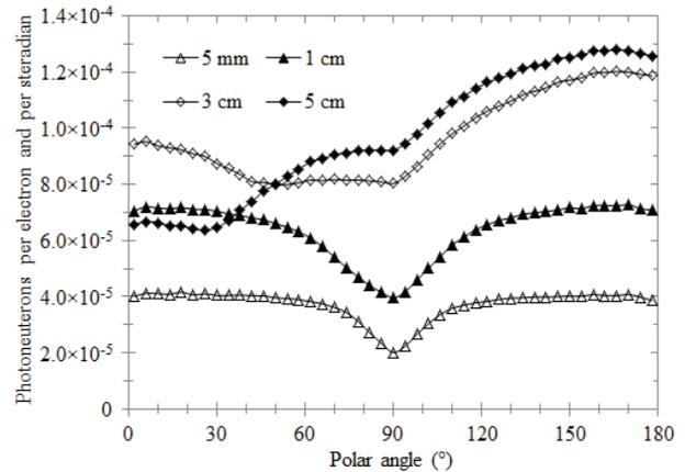
Figure 6: Angular distribution of the photoneutron flux emitted by a tantalum target irradiated by 17 MeV electrons.
