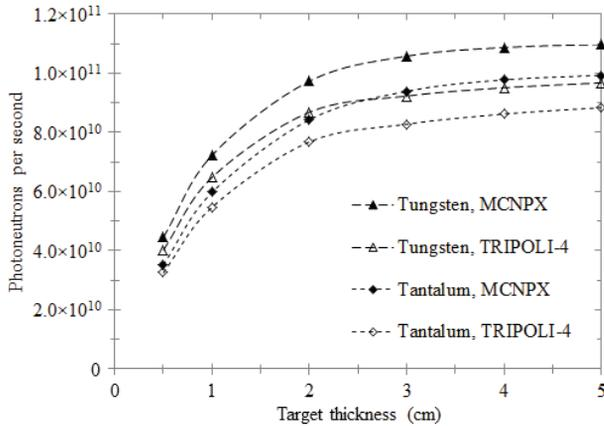
Figure 4: Average emission intensity of the photoneutron flux emitted by a tantalum or tungsten target irradiated by 17 MeV electrons.
