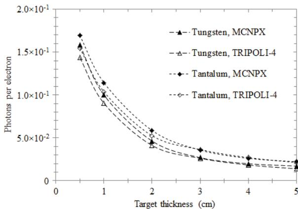
Figure 5: Spurious photon production emitted by a tantalum or tungsten target irradiated by 17 MeV electrons.
