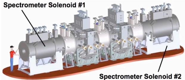
Figure 1: CAD model of MICE cooling channel layout.
