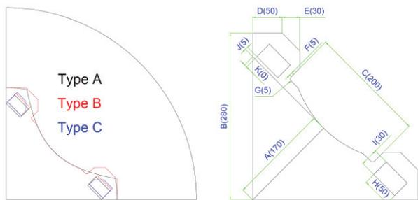
Figure 5: Quadrant cross section of three types of quadrupole magnet (left) and the pole geometry of type B (right).
