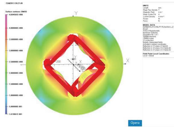
Figure 3: A 3D model of the HTS quadrupole magnet.
