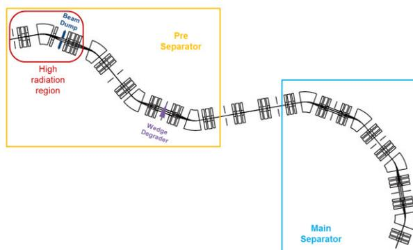
Figure 1: Schematic layout of the fragment separator.
