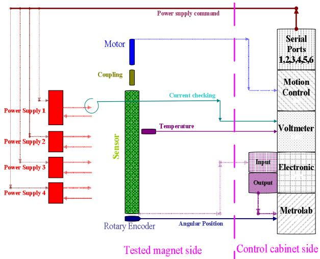
Figure 2: Measurement coil schematic diagram.
