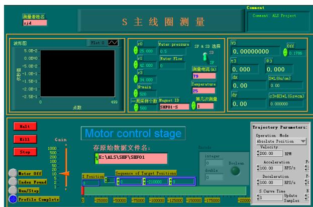
Figure 3: The main measurement menu interface of the control and data acquisition software.
