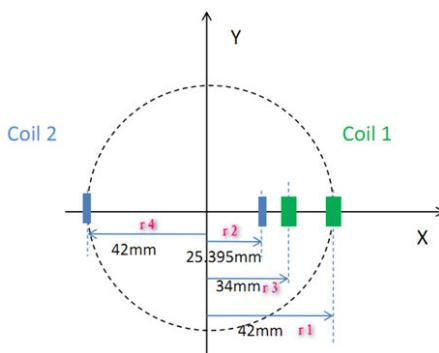
Figure 1: Measurement coil schematic diagram.
