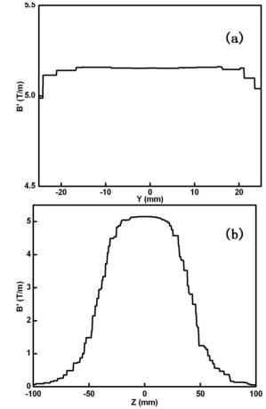
Figure 8: The distribution of magnetic field gradient B' along Y axis (a) and Z axis (b).
