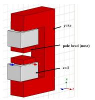
Figure 2: The magnetic model of dipole. 07 Accelerator Technology and Main Systems T09 Room-temperature Magnets
