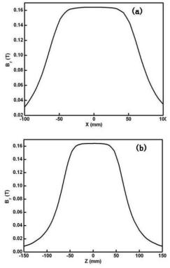
Figure 4: The distribution of  $B_y$  along X axis (a) and Z axis (b).
