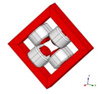
Figure 6: The magnetic model of quadrupole.
