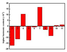
Figure 5: The higher harmonic content of  $B_{y}$  along X axis.
