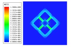
Figure 7: The distribution of magnetic flux on XY cross section of quadrupole.
