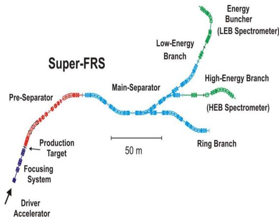
Figure 1: Layout of Super-FRS.
