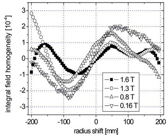
Figure 3: Measured field quality of Super-FRS dipole at various field levels.
