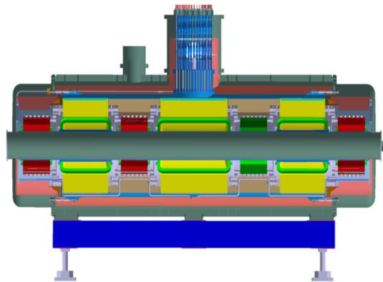
Figure 4: Cross section of biggest multiplet. Yellow and Green are the three quadrupoles (the bigger type 4 in the center), red are the sextupole magnet and green is a steerer magnet. Together with the two octupole coils embedded in the shorter quadrupoles and not shown here, the multiplet contains 9 magnets, which are all powered individually.
