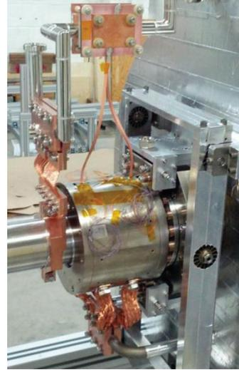
Figure 1: Photograph of the HTS solenoid mounted in the final setup at SRC before insertion into the cryostat.
