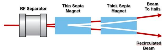
Figure 2: Separator and Septas (not to scale).
