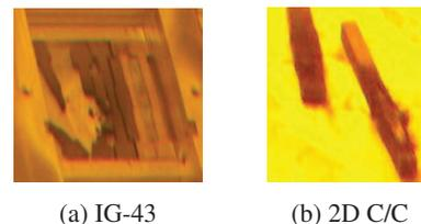
Figure 1: Irradiation induced structural damage by 200 MeV protons at BLIP [1].
