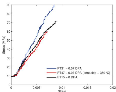
Figure 5: Annealing effect on tensile properties of POCO.
