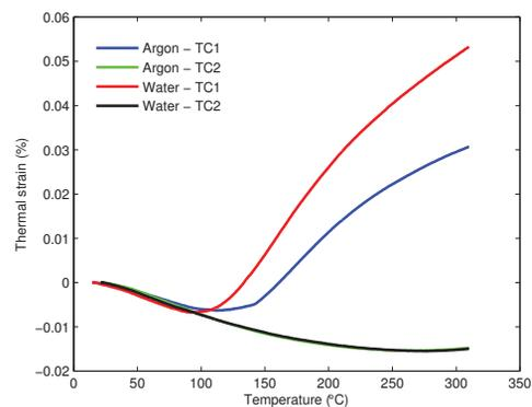
Figure 3: Thermal cycling following irradiation of 3D C/C composite specimens.
