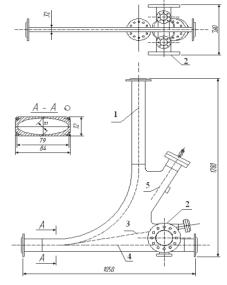
Figure 2: Dipole magnet vacuum chamber drawing.
