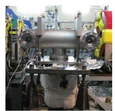
Figure 5: NESTOR inflector vacuum chamber before installation.
