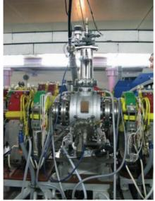
Figure 4: NESTOR RF cavity installed in the ring.
