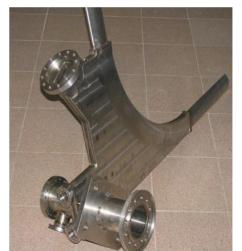
Figure 3: Dipole magnet vacuum chamber view.
