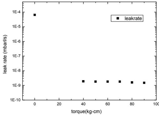
Figure 3: Leak rate vs torque of a diamond-edge gasket
