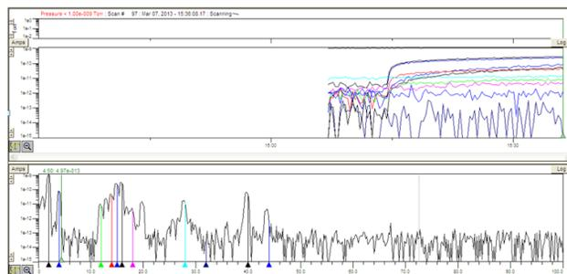
Figure 7: Spectrum of residual gases
