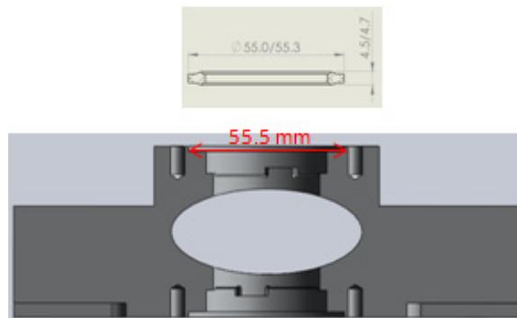
Figure 2: Geometry of the gasket and mating chamber
