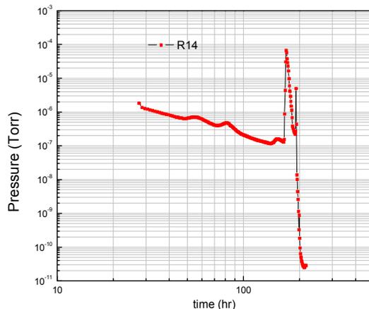
Figure 6: TPS, one cell pumping curve
