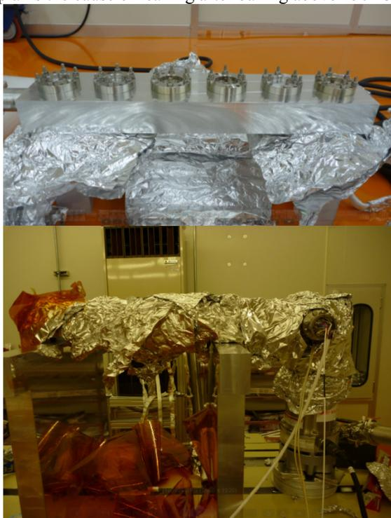
Figure 1: Baking system for Beam Position Monitor
