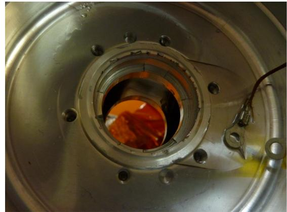
Figure 5: Gasket become severely stuck with the chamber through the baking test
