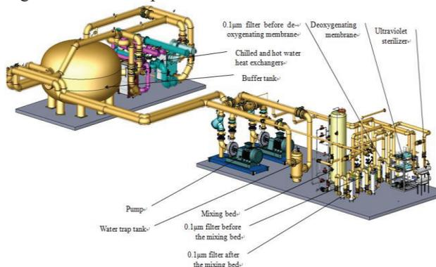
Figure 5: Process of DIW treatment.
