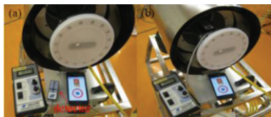
Figure 5: Shielding test of the DCCT assembly.
