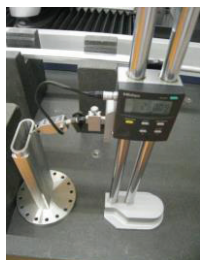
Figure 3: Measurement status after welding.
