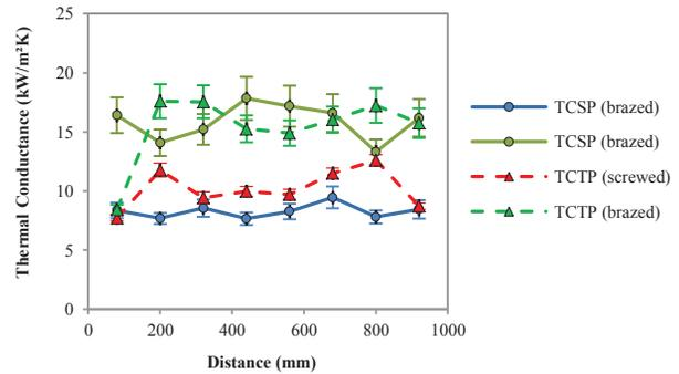
Figure 9: Thermal conductance of four different jaws.
