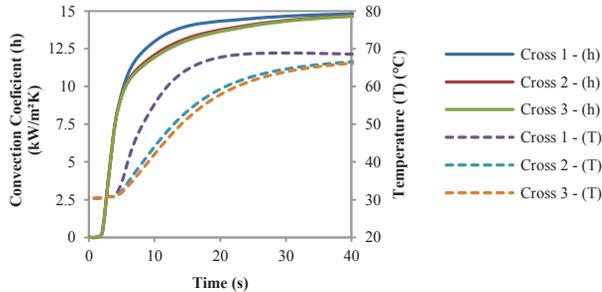
Figure 7: Typical boundary conditions for the 2D model of one tube in one section.
