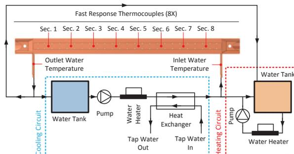
Figure 5: Simplified schematic of the hydraulic circuit.
