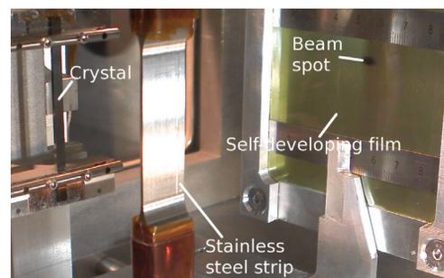
Figure 2: Snapshot captured with the webcam during the measurements, showing the crystal mounted on the aluminium holder (left), the stainless steel strip used during the alignment (center) and the self-developing film (right) with the beam spot being visible as black area.
