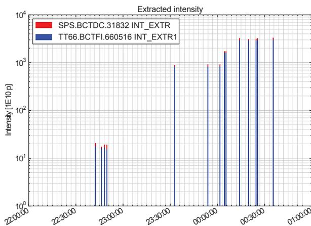
Figure 4: The extracted beam intensity as measured in the SPS and in the HiRadMat beam line.
