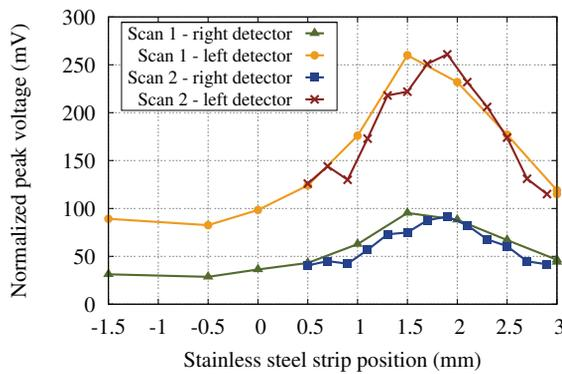
Figure 3: Examples of position scans aiming to align the target with respect to the beam.
