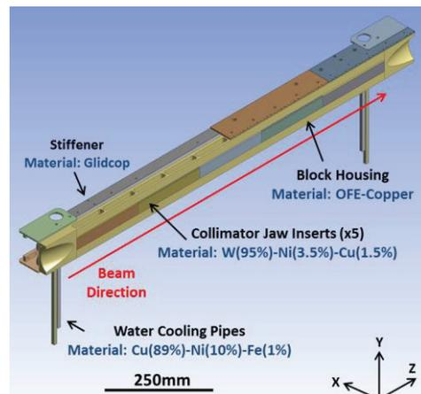
Figure 1: Left jaw assembly of a TCTH.
