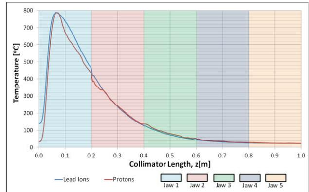
Figure 4: Temperature peak profiles within the jaw inserts along the beam direction for ions and protons.
