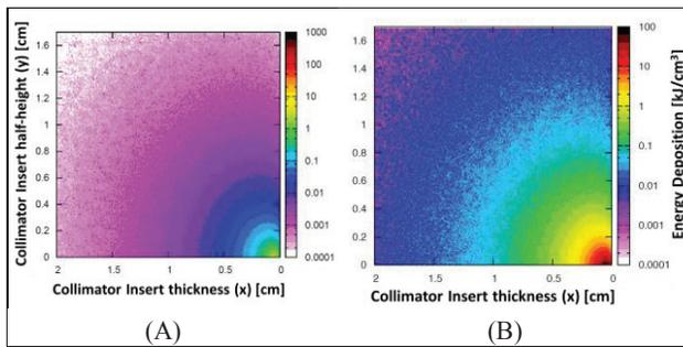
Figure 2: Energy deposition cuts in the x-y plane at the location of  $T_{\max}$  in z. (A) 1 nominal bunch of lead ions ( $7 \times 10^7$  ions, 2759 GeV/n) with  $T_{\max}$  occurring at  $z = 6.5$  cm. (B) 1 nominal bunch of protons ( $1.15 \times 10^{11}$  p) at 7TeV with  $T_{\max}$  occurring at  $z = 7$  cm.
