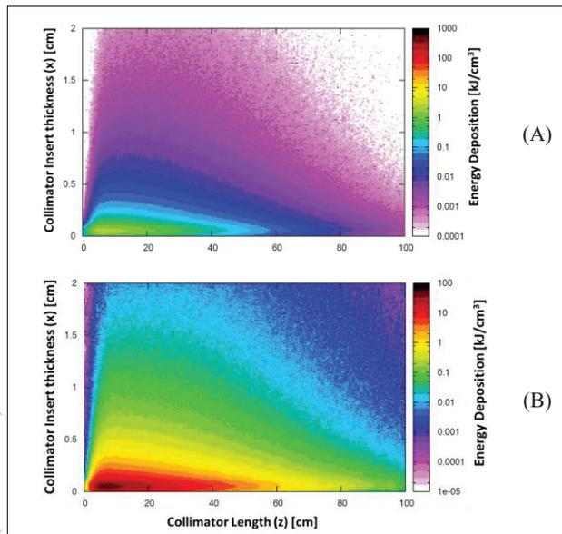
Figure 3: Energy deposition cuts in the x-z plane at collimator insert half-height (plane of symmetry). (A) 1 nominal bunch of lead ions ( $7 \times 10^7$  ions, 2759 GeV/n). (B) 1 nominal bunch of protons ( $1.15 \times 10^{11}$  p) at 7TeV.
