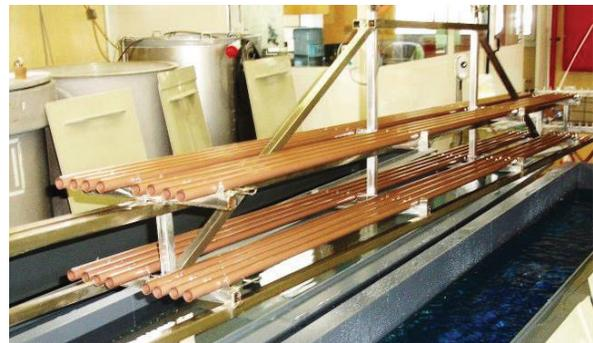
Figure 1: Series etching of the extruded copper tubes.
