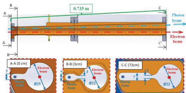
Figure 6: Vessel with antechamber.
