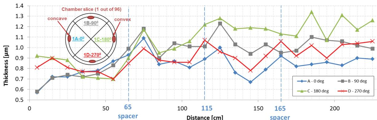
Figure 5: XRF NEG-coating thickness distribution measurement results of the 3 degrees bent vacuum chamber.
