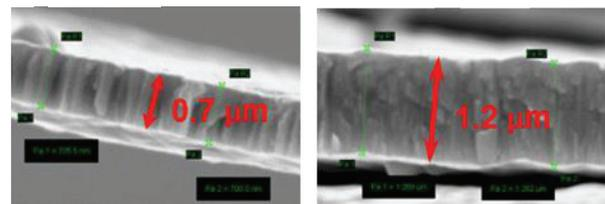
Figure 4: NEG film thickness measurement by SEM.
