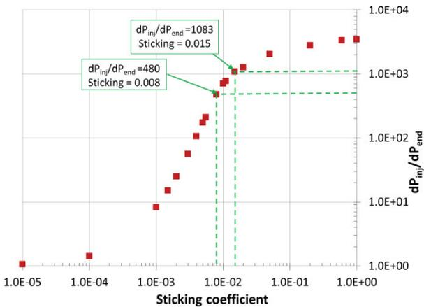
Figure 2: Monte Carlo simulations results for a 1 m long NEG-coated tube of 21 mm inside diameter.
