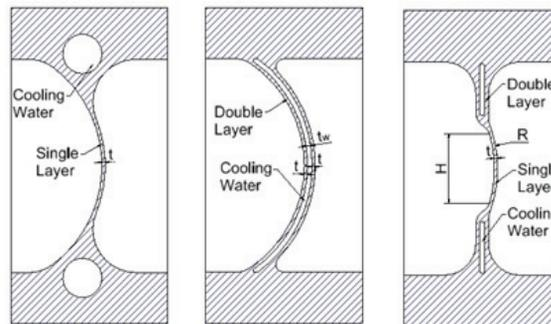
Figure 1: Section views of three structures (L: Single layer structure; M: Sandwiched structure; R: Single-Double Layer Structure).
