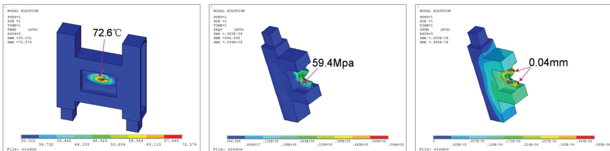
Figure 4: Thermal-stress results of modified structure(L: temperature; M: Von Mises stress; R: displacement).
