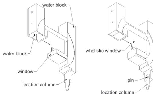
Figure 2: The modification of PBW (L: original design; R: modified design).
