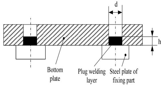
Figure 3: Draft of plug welding.
