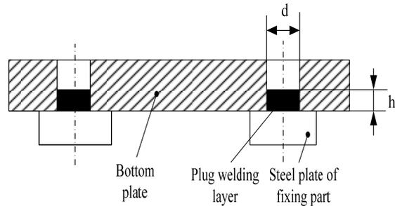
Figure 3: Draft of plug welding.
