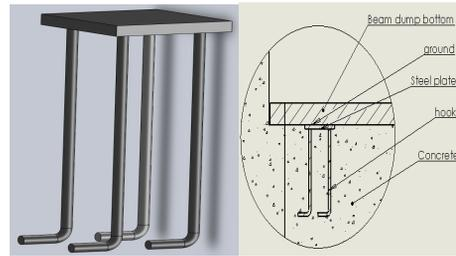
Figure 1: Structure of Fixing Part and its Installation.
