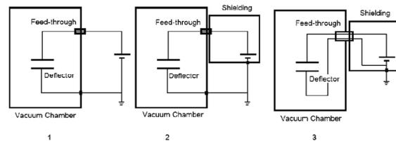
Figure 8: Improvement made for electromagnetic shielding.
