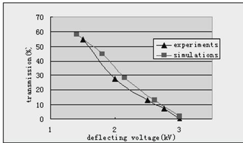
Figure 6: The simulations and experiments results of the deflecting voltage versus RFQ transmission.
