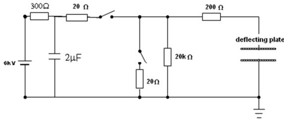
Figure 4: The schematic layout of the chopper circuit.
