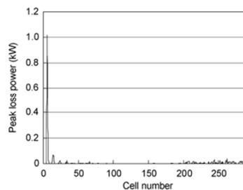
Figure 3: The lost pulse beam power versus the RFQ cell number.
