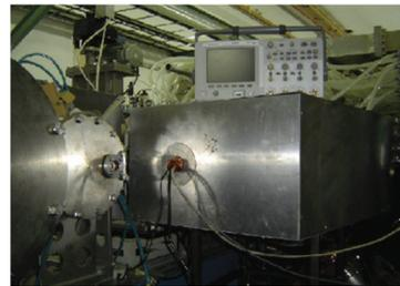
Figure 7: The aluminium rack for electromagnetic shielding.
