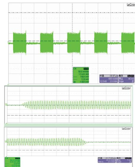
Figure 5: Beam signal of the BPM. Left: 500ns/div right: 20 ns/div.
