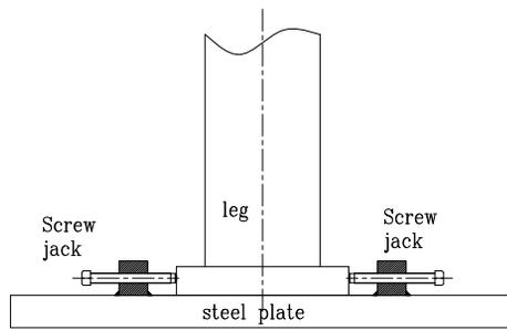
Figure 7: Adjusting the azimuth position.
