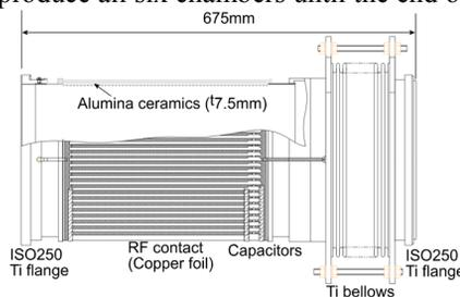
Figure 7: Outline view of the alumina ceramics duct for the quadrupole corrector.
