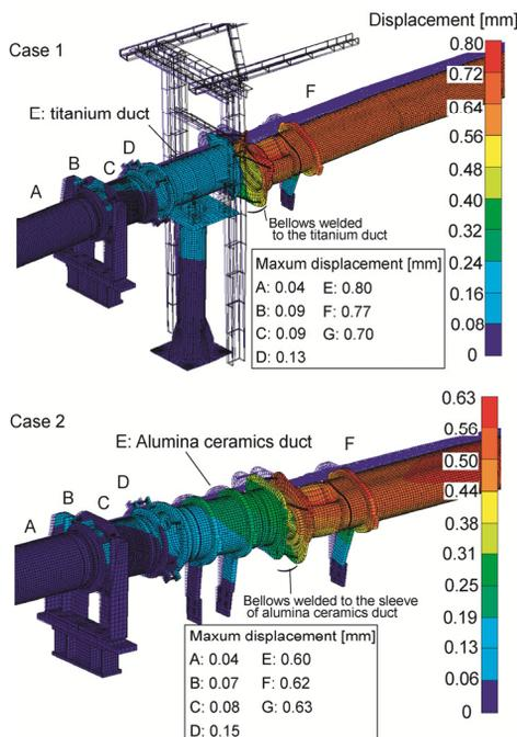
Figure 6: The contour figures of the displacements. Symbols A-G correspond to the equipments in Fig. 5.
