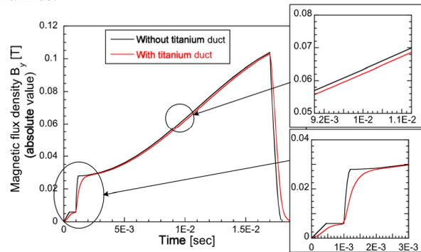
Figure 3: Time response of the magnetic flux density with and without the titanium duct at  $(x,y,z)=(100,0,0)$ .
