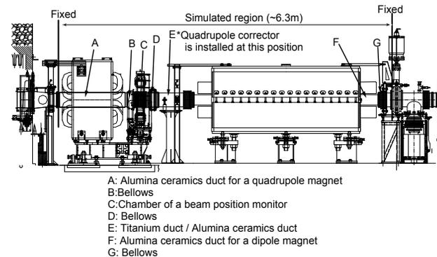
Figure 5: The region and equipments of RCS beam line, which are simulated for the structure analysis.
