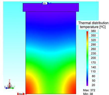
Figure 4: Calculation results of the temperature distribution for the titanium duct at thermal equilibrium.
