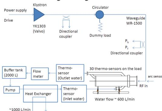
Figure 4: High-power test setup and arrangement.
