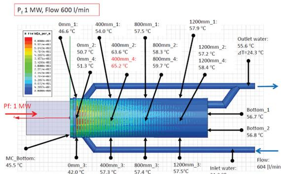
Figure 6: Thermo-sensors response at 1 MW input.
