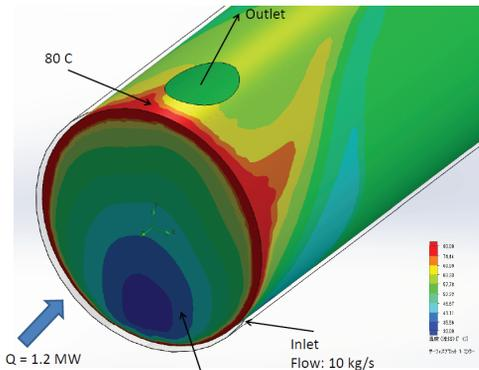
Figure 8: Temperature distribution in the load with dummy heat load (1.2 MW).
