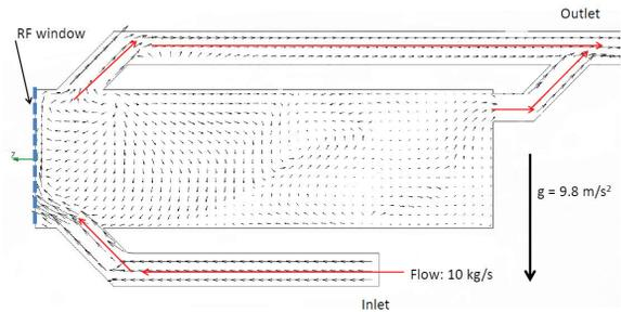
Figure 7: Velocity vector of water-flow.
