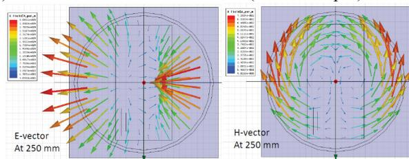
b) E-field (left) and H-field (right) distribution on the cross section at 250 mm away from the rf window.
