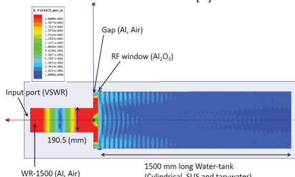
a) Calculation model with E-field (1.2 MW input)
