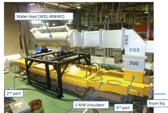
Figure 1: Picture of the cylindrical-type water-load mounted on the 3<sup>rd</sup> port of the 1 MW circulator.
