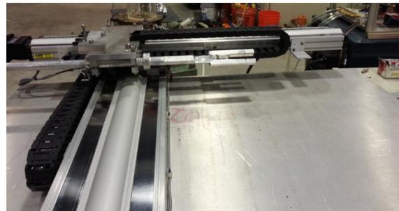
Figure 1: The Hall probe on a 2D translation stage.
