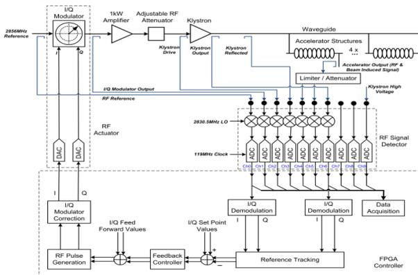
Figure 8: Architecture of the LLRF Firmware.
