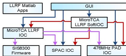
Figure 7: Architecture of the LLRF firmware/software.
