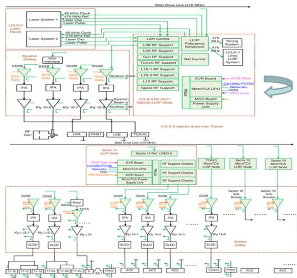
Figure 2: The overview of the LCLS-II LLRF Control System.
