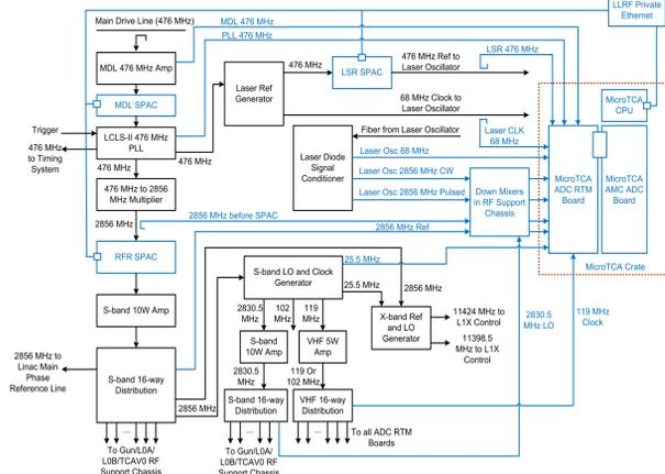
Figure 3: LLRF Frequency Reference Subsystem [2].
