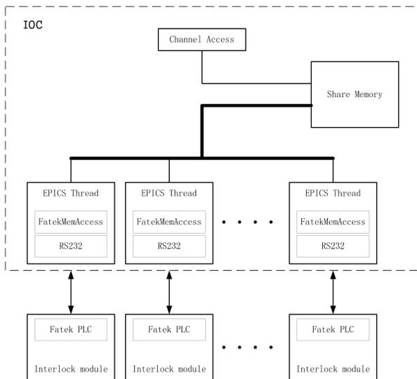
Figure 2: structure of interlock monitoring & temperature change rate monitoring IOC.
