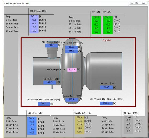
Figure 3: EPICS medm display of SRF temperature change rate monitoring module.
