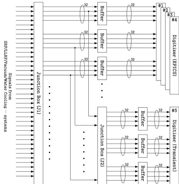
Figure 1: The hardware structure of data acquisition.
