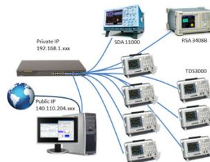
Figure 9: Data acquisition setup of automatic logging tools.
