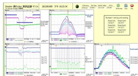
Figure 5: Bumper 3 missing fire event pattern in “Booster and kicker recorder”
