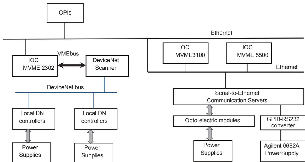
Figure 2: Layout of the SDUV-FEL power supply control system.
