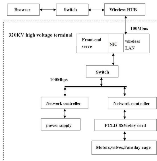
Figure 1: Connection diagram of the control system.
