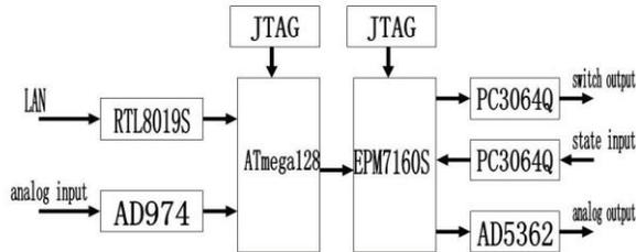
Figure 2: Hardware circuit block diagram.
