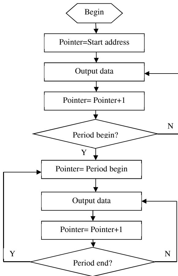
Figure 3: Algorithm of data output.
