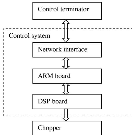
Figure 1: Structure of hardware platform.
