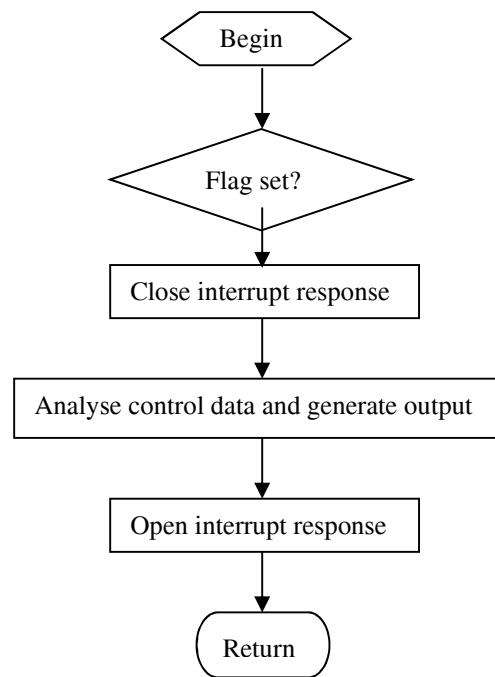
Figure 2: Algorithm of generating output data.
