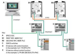
Figure 1: Redundant control system.
