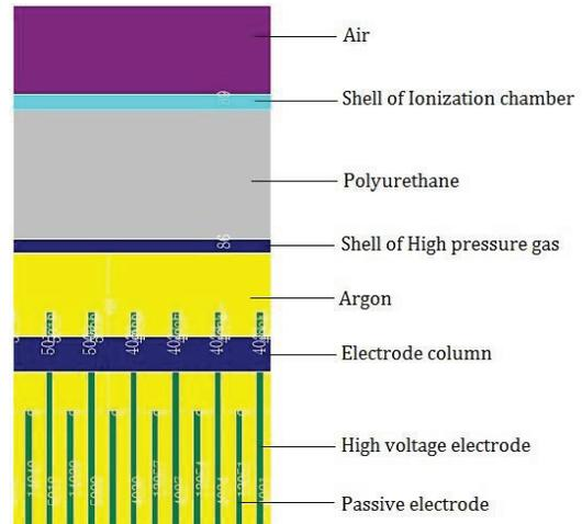
Figure 2: Center section of ionization chamber perpendicular to the electrode.
