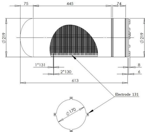
Figure 1: The schematic diagram of the ionization chamber.
