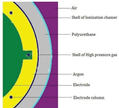
Figure 3: Section of any electrode plate parallel to electrode.
