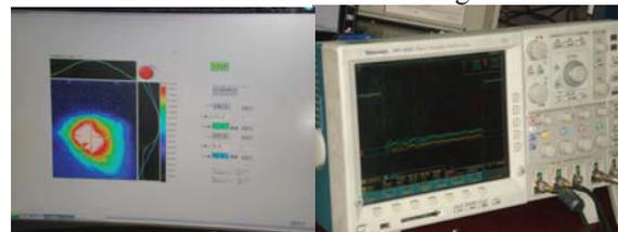
Figure 7: Electron beam profile and pulse at the exit of the first accelerating section.
