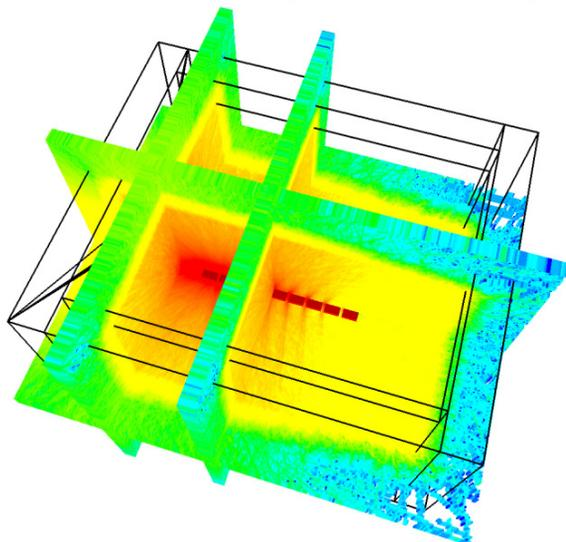
Figure 6: Perspective view of mesh tally planes. Total DE from simulation is superimposed onto mesh planes.
