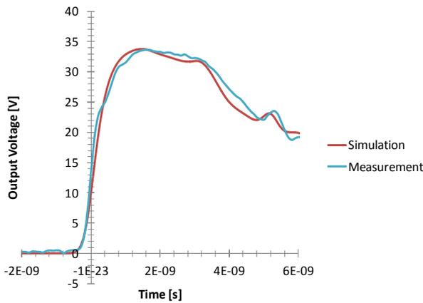
Figure 2: Single dipole output voltage temporal profile.
