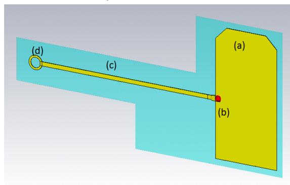
Figure 1: Single dipole model: (a) a capacitor, (b) switches, (c) transmission line, (d) equilibration rings.
