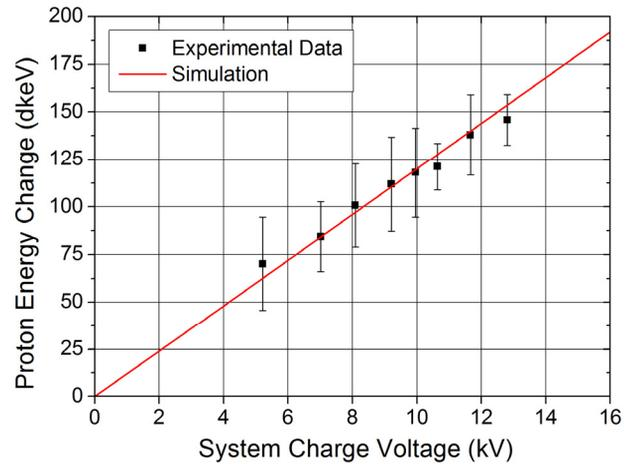
Figure 5: Experimental Data and Simulation Results for proton energy change as a function of system charge voltage for a short accelerator section.
