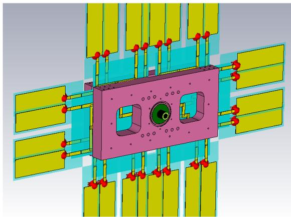
Figure 3: A DWA system model with 24 dipoles.
