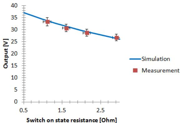
Figure 4: Total output voltage of the 24 dipole system.
