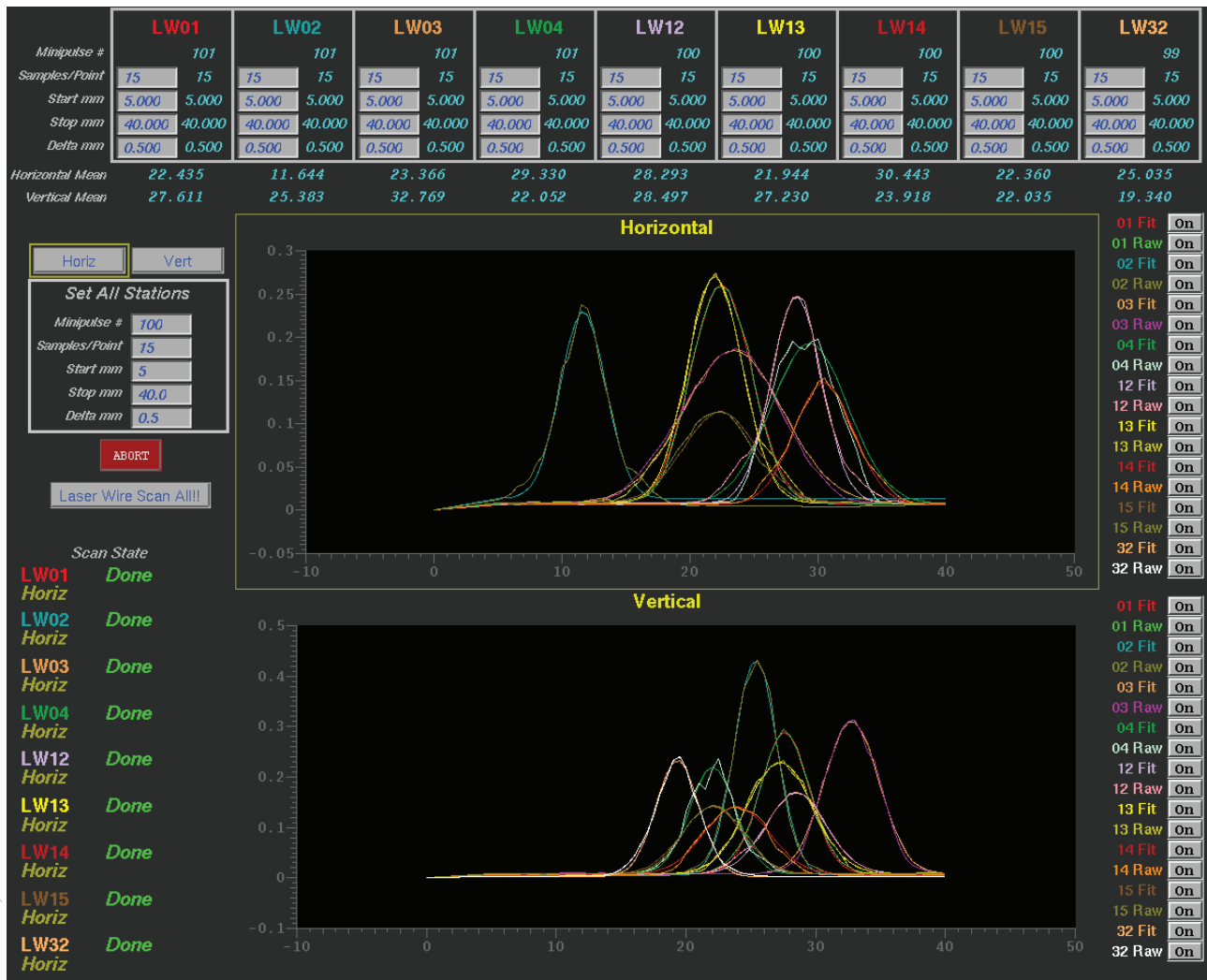
Figure 3: EDM screen of the laser wire based parallel profile scan. The EDM screen provides the user with the ability to change settings for either all of the laser wire stations or individual stations. Prominently displays the horizontal and vertical profiles for each station on the same plot, which axis is selected, and the state of the scan. For convenience, toggle buttons along the side of the plot enable/disable the display of individual profiles.
