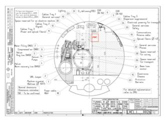
Figure 2: Typical LHC tunnel cross section with indication of the position for the LHeC magnets.
