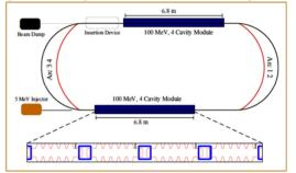
Figure 10: Schematic layout of an ERLTF at CERN [11].
