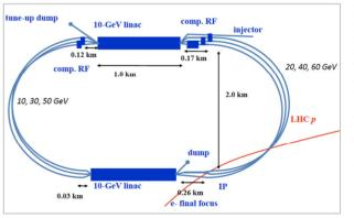
Figure 4: Schematic layout of the 60 GeV ERL option.
