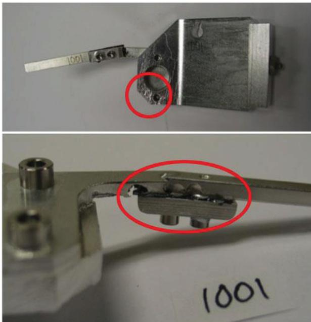
Figure 5: Photos of a failed stripper foil bracket showing reflected convoy electron damage (top) and arcing damage (bottom). (Photos reproduced from Ref. [10])
