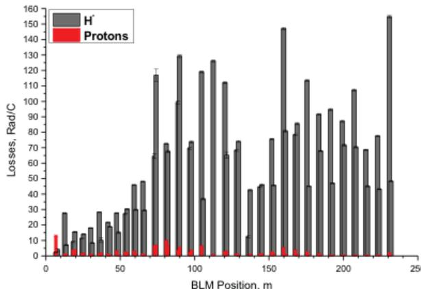
Figure 1: Beam loss monitors along the SCL, showing the proton (red) vs.  $H^-$  (grey) beam loss for the design optics case, for 30 mA beam current.
