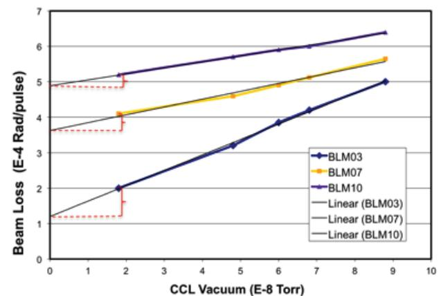
Figure 3: Beam loss in the Oak Ridge SCL as a function of gas pressure in the last CCL tank. The nominal gas pressure is  $\sim 2 \times 10^{-8}$  Torr, and the red brackets indicate the beam loss due to residual gas stripping during nominal operations.
