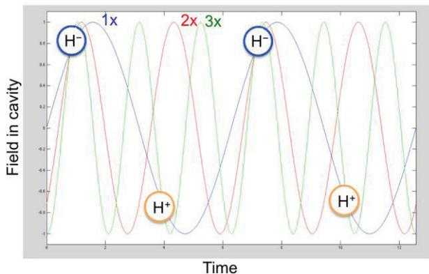
Figure 2: Electric fields in a linac for three different frequencies.
