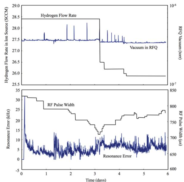
Figure 4: Example of Oak Ridge RFQ resonance error being controlled by automatic RF pulse width adjustments. Top: the hydrogen gas flow rate in the ion source is reduced midway through the plot. Bottom: In response to the drop in flow rate the RF pulse width is automatically increased and the resonance error becomes more stable. (Figure reproduced from ref. [7])
