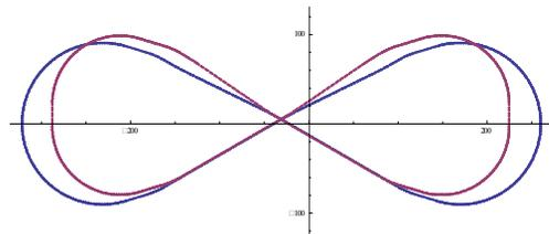
Figure 1: This overlay shows footprints of the original (in purple color) and the new (in blue color) booster rings.
