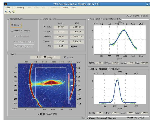
Figure 2: The beam size and beam center measurements on the screen located at the high dispersion region behind the bending magnet were performed for calculating the energy spread and energy variation of the 150 MeV LINAC.
