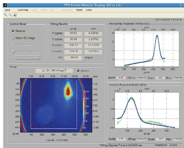
Figure 1: The beam size measurements on the screen after the quadrupole triplet and before the bending magnet were performed for calculating the Twiss functions and emittance of the 150 MeV LINAC.
