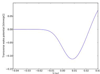
Figure 2: Short range geometric wake field of the cavity BPM used at ATF for a Gaussian shaped bunch length with standard deviation of 7mm.
