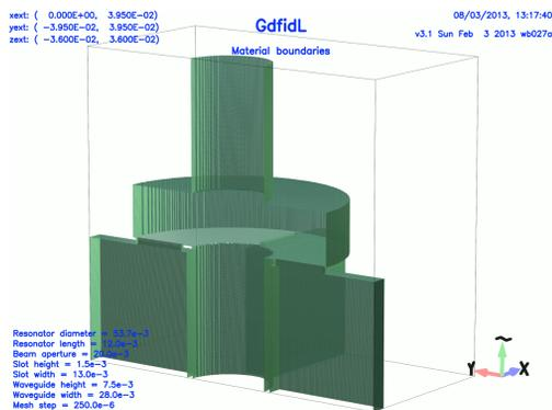
Figure 1: Geometry of the cavity BPM used at ATF.
