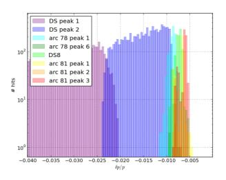
Figure 6: Distributions of the  $\delta p/p$  of the particles lost in the main peaks downstream IR7, grouped by peak. The names are arbitrary. There is a clear limit of  $\delta p/p$  under which the particles are lost.
