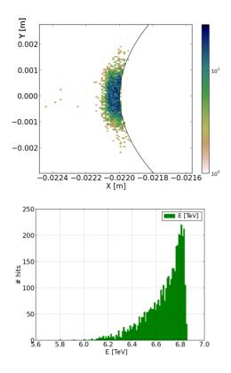
Figure 5: Transverse (top) and energy (bottom) distribution of the losses corresponding in the first peak in the dispersion suppressor right of IR7: 20270 m < s < 20350 m. The black circle represents the aperture of the arc. The highest energy for a lost particle is 6.86 TeV, giving  $\delta p/p = -0.02$ .
