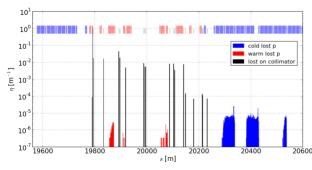
$\odot$  Figure 3: Horizontal loss map for IR7. Every peak in the  $\Xi$  DS corresponds to a maximum of the dispersion.
