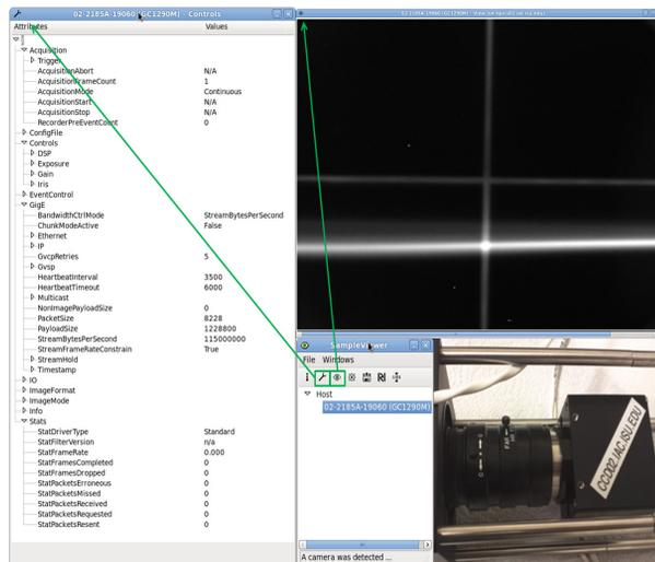
Figure 2: This is SampleViewer and the Prosilica GC1290 GigE CCD camera with the attached lens.
