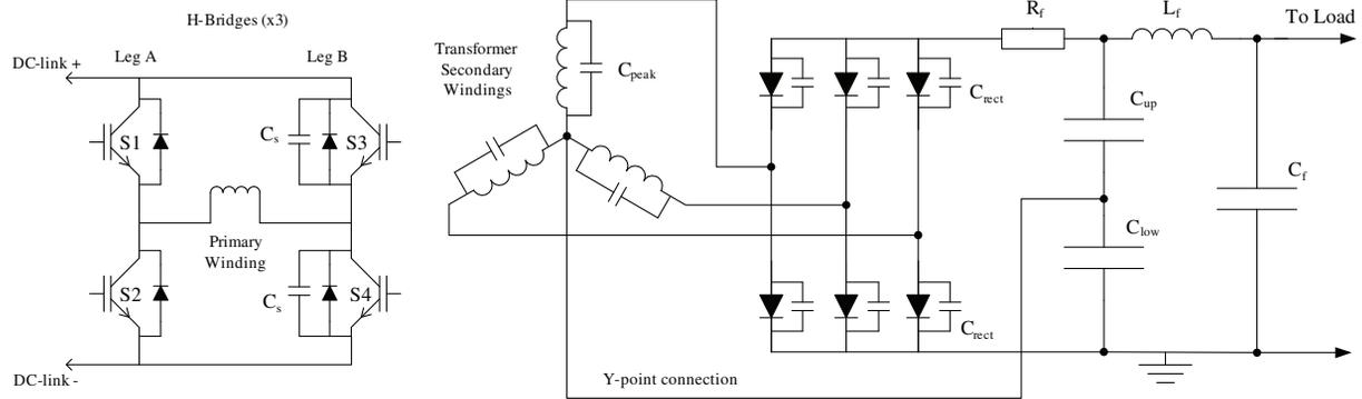
Figure 1: Simplified schematic of a typical HVCM. The primary windings of the three H-Bridges, shown on the left, are connected to the secondary windings in a 'Y' shown on the right.
