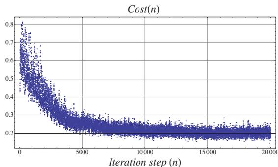
Figure 5: A less noisy cost was detected in the computer in  $n = 20,000$  steps when each iterative extremum seeking step calculated the cost based on the average of 10 HVCM shots with fixed settings.
