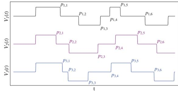
Figure 2:  $p_{i,j}$  is the  $j^{\text{th}}$  switching edge of the  $i^{\text{th}}$  drive waveform  $V_i$  of each of the three input H-Bridges (as shown in Figure 1). The extremum seeker tunes only the first 8 switching edges of each drive waveform, which influence the rise time. The other waveforms are maintained at pre-calculated values.
