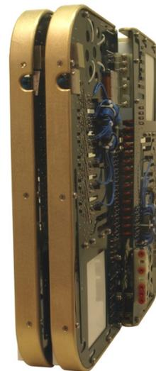
Figure 3: Stack of four connected modules viewed on edge. Fifty of these modules are shown connected in Figure.
