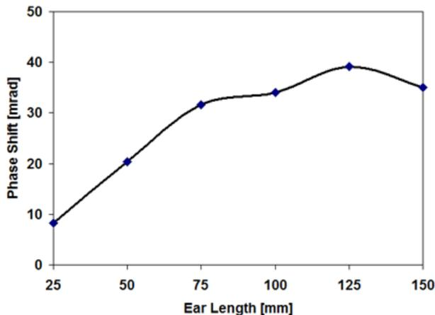
Figure 4: Saturated phase-shift versus ear-length graph (carrier signal:  $f = 1.5224$  GHz,  $\pi$ -mode).
