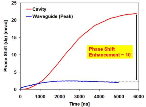
Figure 2: Phase shift versus time graphs of waveguide (blue) and cavity (red) beam pipe models. The cavity enhances the phase-shift by a factor of 10. (ear length/width = 60 mm/6mm)
