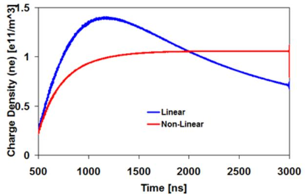
Figure 3: Electron cloud charge density versus time graphs from two different assumptions on the wave traveling distance in the cavity: linear- (blue) and non-linear (red) increases.
