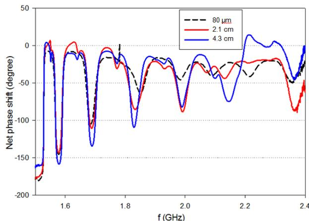
Figure 5: Saturated phase-shift versus ear-length graph (carrier signal:  $f = 1.5224$  GHz,  $\pi$ -mode).
