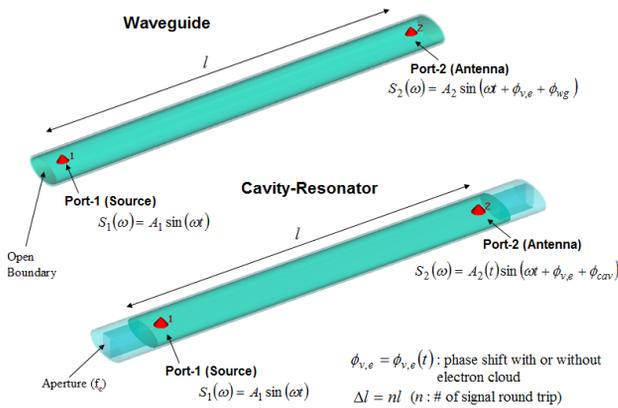
Figure 1: Finite-integral-technique (FIT) simulation models (a) elliptical waveguide and (b) elliptical cavity.
