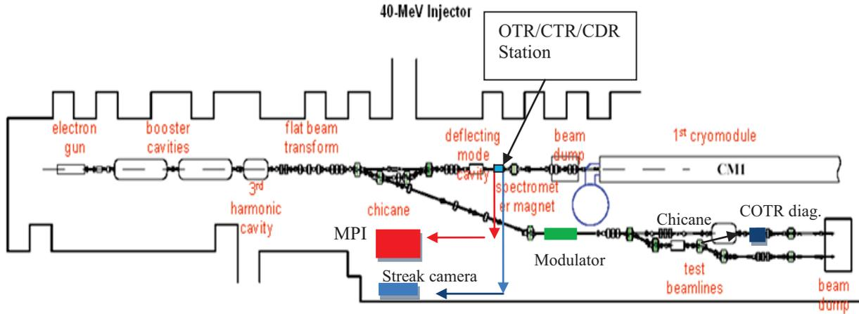
Figure 1: Schematic of the injector for the ASTA facility showing PC rf gun, booster accelerators, and beamlines. (courtesy of M. Church). The locations of the streak camera and MPI are also indicated.
