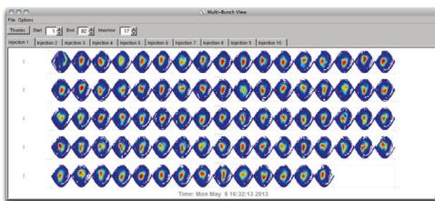
Figure 3: Full batch window showing reconstructions of Booster batch upon injection into the Main Injector.
