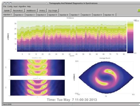
Figure 2: One possible layout for the main window showing an emittance plot (top), average bunch reconstruction (lower right), projection of reconstruction (middle left), and average input data (lower left). Another can be seen in fig. 1
