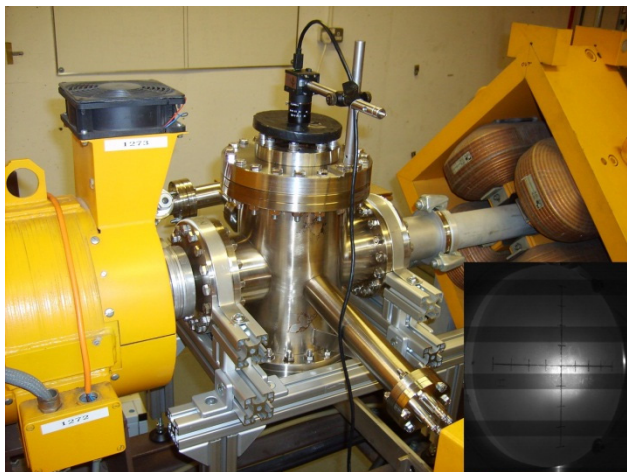
Figure 2: Experimental vessel integrated into the beam line in the accelerator vault (in the right bottom corner of the picture – image of the scintillating screen with marked axes for relating physical dimensions to distances on the image).
