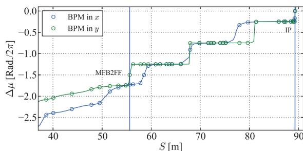
Figure 2: ATF2 horizontal and vertical betatron phase  $\mu$  compared to the IP phase.
