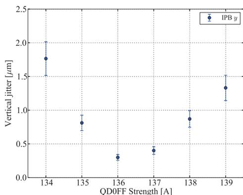
Figure 7: IP waist position scan, around IPB, using QD0FF current.
